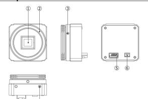
① IMAGE SENSOR FRONT FACE The light receiving face of the image sensor
